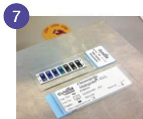
7 Check the temperature of the hotplate using the slide surface thermometer provided. Denature the slide/device at 75°C for 2 minutes.
