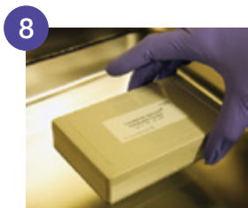
8 Place slide/device in hybridisation chamber supplied and float on the surface of a clean 37°C waterbath overnight.
